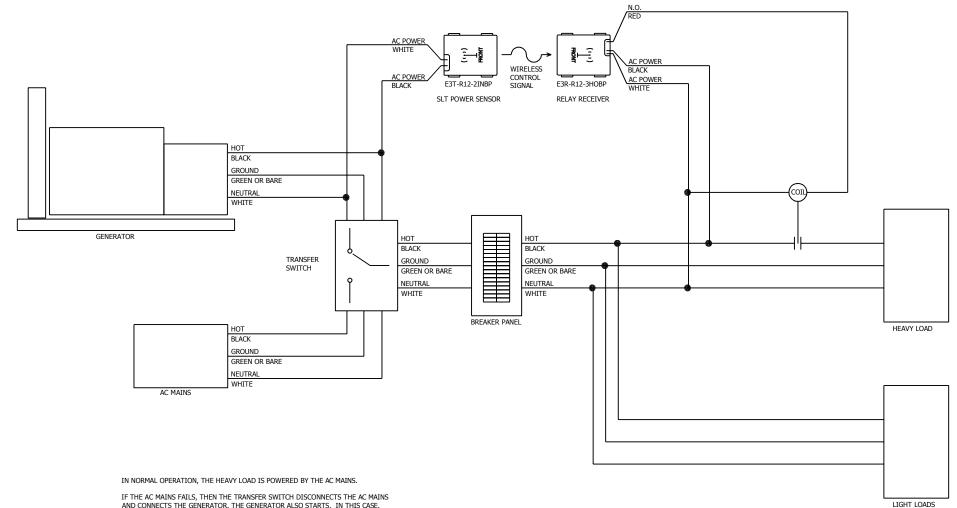
IF THE AC MAINS FAILS, THEN THE TRANSFER SWITCH DISCONNECTS THE AC MAIN: AND CONNECTS THE GENERATOR. THE GENERATOR ALSO STARTS. IN THIS CASE, THE GENERATOR IS TOO SMALL TO RUN THE HEAVY LOAD, BUT IS FULLY CAPABLE OF RUNNING THE LIGHT LOADS.
