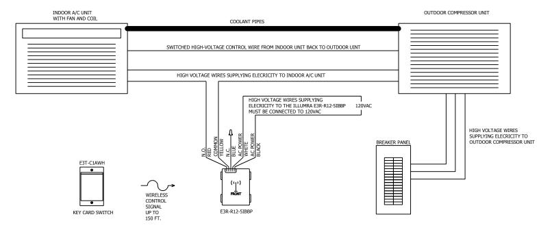
WHEN GUEST ARRIVES IN THEIR ROOM, THEY INSERT THEIR KEY CARD INTO THE KEY CARD SWITCH. THE KEYCARD SWITCH TRANSMITS A CONTROL SIGNAL TO THE WIRE-IN RELAY, WHICH ACTIVATES THE INDOOR A/C UNIT.
