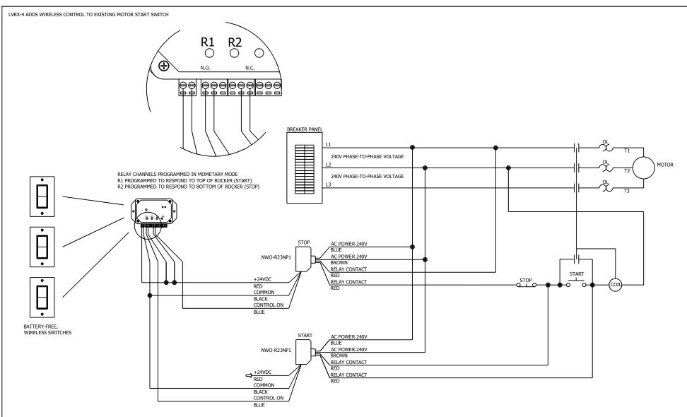
MOTOR STARTS BY PRESSING START SWITCH OR BY PRESSING THE TOP HALF OF ROCKER ON ANY WIRELESS SWITCH.
