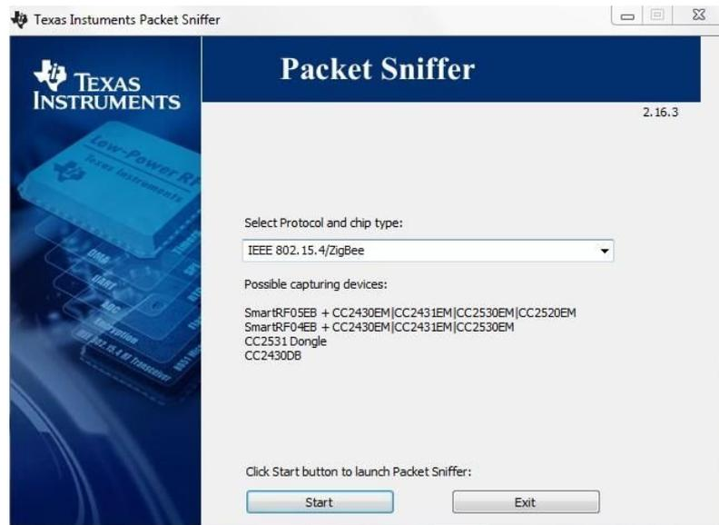
**Figure 17 – Protocol selection dialog of TI SmartRF Packet Sniffer**
