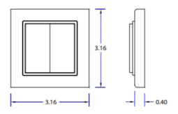
For flush mount, mount the switch without the backplate into either a standard electrical switch box or a low voltage mounting bracket using included screws.
