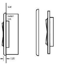
For flush mount, mount the switch without the backplate into a standard electrical switch box using included screws.
