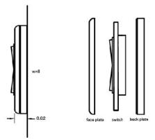
For surface mount, attach included backplate to the wall using screws or adhesive.
